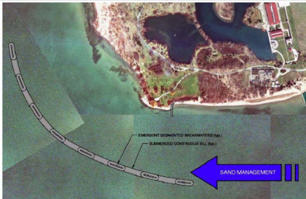
Figure 2. Representation of the offshore protection to be explored during the detailed design process, showing emergent breakwaters connected by an underwater sill in plan view. Source: Shoreplan Engineering Limited, 2007.
