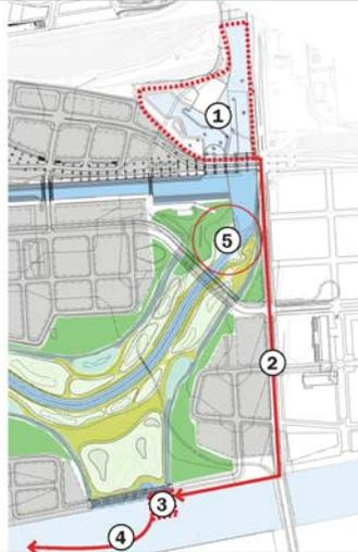
Note: the Ship Channel dewatering facility and hydraulic dredge located in area 1 will be transportable in the event of excessive sediment accumulation over time in the Keating Channel and/or new mouth of the Don.
