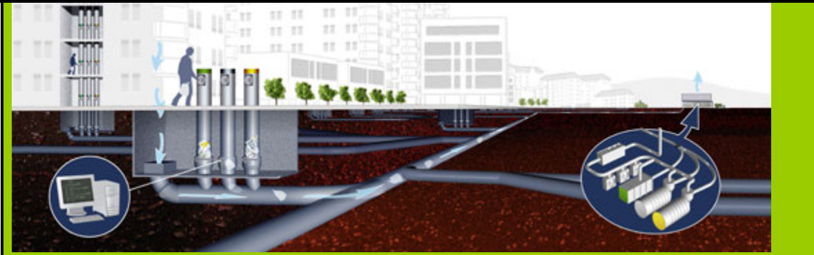
Figure 6.1: Visualisation of Envac Collection System (Source: Envac, 2009)
