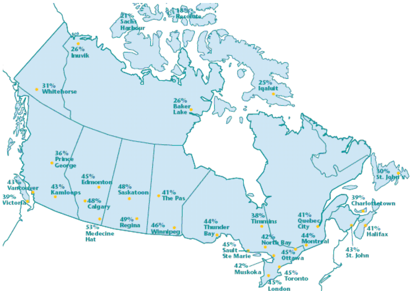
Figure 3.1 Potential contributions of solar water heaters to energy for water heating in different Canadian cities. (Assumes a freeze-protected system with 6 m 2 single-glazed flat plate solar collectors and two 270 litre hot water tanks; NRCan, 2003b)
